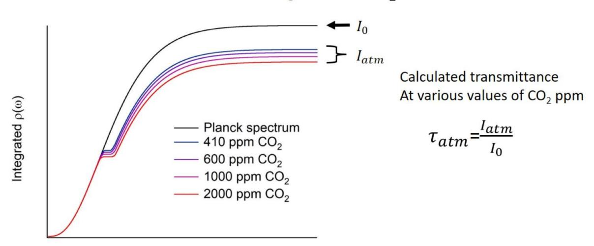
The transmittance calculated for CO<sub>2</sub> only is shown below.
