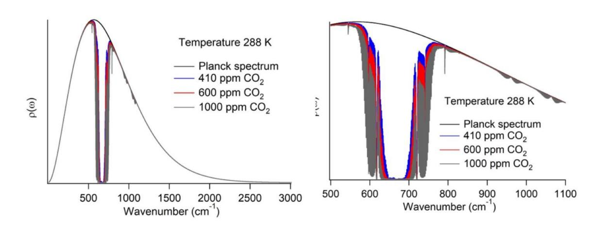
The transmittance of radiation at all frequencies is determined by taking the integral of the Planck function with each of the added transmission regions for CO<sub>2</sub>.
