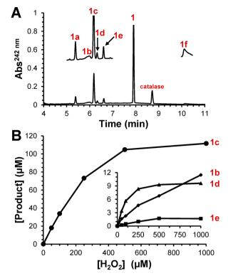
**Figure 2.** (A) HPLC chromatogram of the reaction of 5-Br-indole (500  $\mu$ M) with DHP B (10  $\mu$ M) in the presence of H<sub>2</sub>O<sub>2</sub> (500  $\mu$ M) at 25 °C (5% MeOH in 100 mM KP<sub>i</sub>, pH 7). The reaction was quenched upon addition of catalase and subjected to HPLC analysis as described in the text. (B) Product distribution for the reaction described in panel A under variable [H<sub>2</sub>O<sub>2</sub>].
