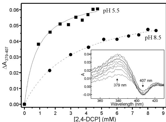
Fig. 3. Correlation plots of absorbance changes ( $\Delta A$ ) versus 2,4-DCP concentration at pH 5.5 and 8.5; the corresponding optical difference spectra are reported in the inset.
