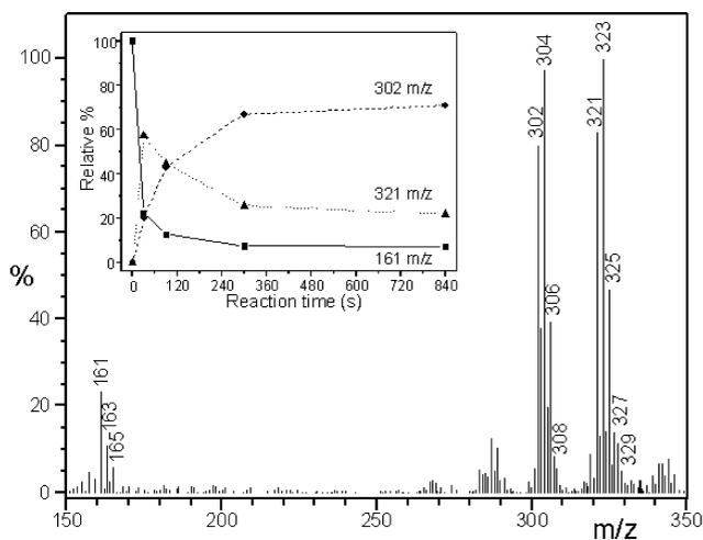
Fig. 4. Mass spectrum of the reaction mixture  $H_2O_2/HRP/2,4-DCP$  after 90-s incubation; the time-dependence of the relative intensity of 161, 302 and 321  $m/z$  peaks is reported in the inset.
