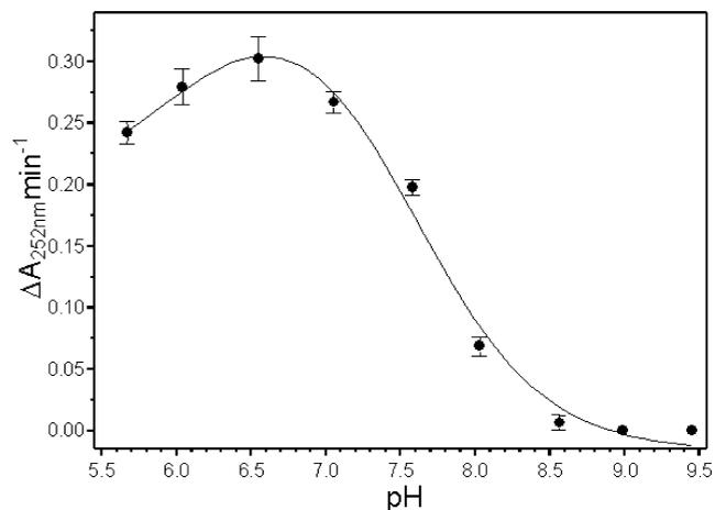
Fig. 2. pH-dependence of the initial rate of HRP-catalyzed oxidation of 2,4-DCP expressed as absorbance changes at 252 nm.
