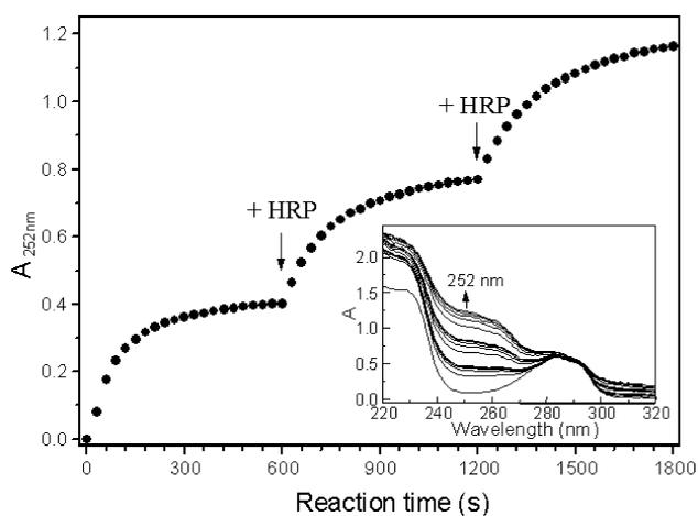
Fig. 1. Absorbance change at 252 nm versus reaction time; arrows indicate further additions of HRP at 600- and 1200-s reaction time. The concurrent evolution of the electronic spectrum is reported in the inset.
