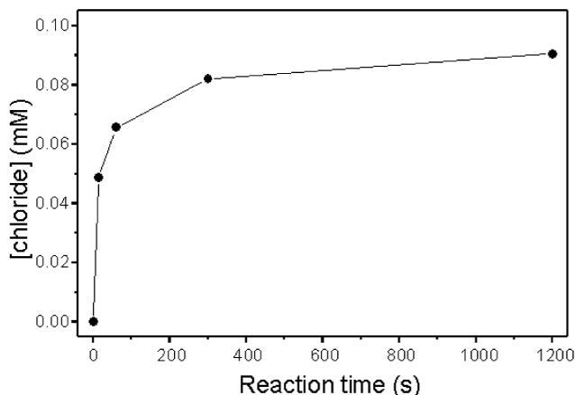
Fig. 5. Time-course of chloride release during the  $\text{H}_2\text{O}_2$ -oxidation of 2,4-DCP catalyzed by HRP. Chloride was detected as chloromercurate(II) complex ion with the indirect analytical method described in the Material and methods section.
