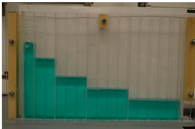
Figure 4. Plastic water-flow device with partitions at the 1st, 3rd, 6th, 10th, and 15th positions to represent steady-state through an atmosphere with diminishing concentrations of a greenhouse gas as a function of altitude.
