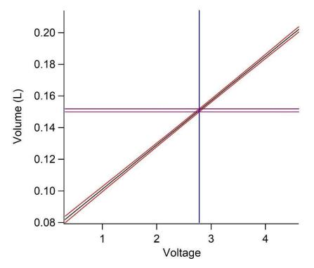
We find  $\sigma_V = 0.0019$  L at the midpoint (or average)..The maximum and minimum volumes are 0.2024 and 0.0824 L, respectively. Given that the calculated volume at the midpoint is 0.150 L, the relative error is approximately 1.3%.
