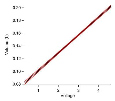
The practical extraction of the 95% confidence limit of the volume can be obtained graphically.
