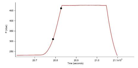
This is shown between the black dots for one of the cycles of compression and expansion. Extract both the pressure and the volume points from 20788 to 20826. Then we use those points to calculate a value of gamma at each point. Analysis of several of the argon data sets was carried out by calculating
