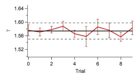
For Ar we obtained an average of  $\gamma = 1.57$ , which corresponds to  $C_v = \frac{7}{4}R$ . Given the 95% confidence limit, it was appropriate to round to three significant figures.
