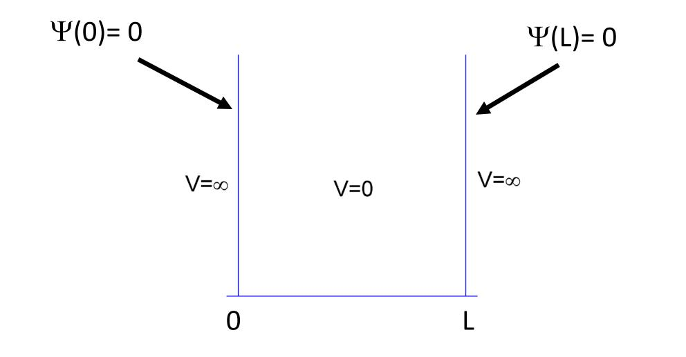
The boundary conditions determine the values for the constants C and D
