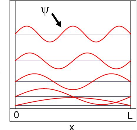
The solutions have increasing numbers of nodes as the quantum number n increases. The lowest solution has no nodes. It is constrained at either end like a guitar string. The lowest solution is like the fundamental of a guitar string.
