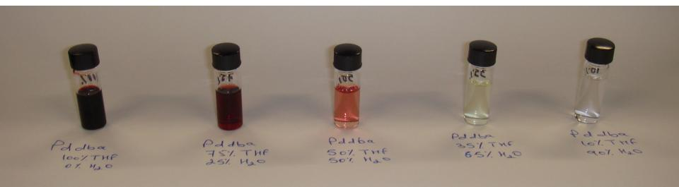
One can measure the spectrum and calculate the concentration of  $Pd_2(dba)_3$  in various solvents to determine the limit of solubility. This organometallic Compound is soluble in THF and insoluble in water.
