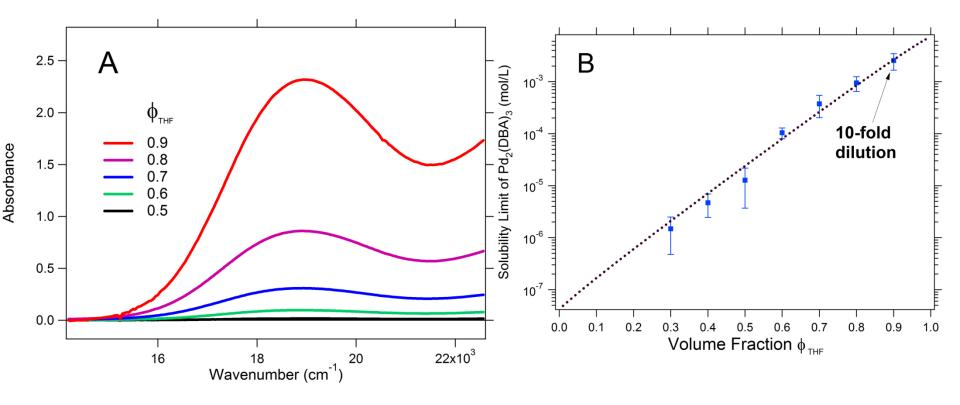
Analysis can use absorption spectrometry. However, to determine the calculation using the absorption spectrum one needs the extinction coefficient.
