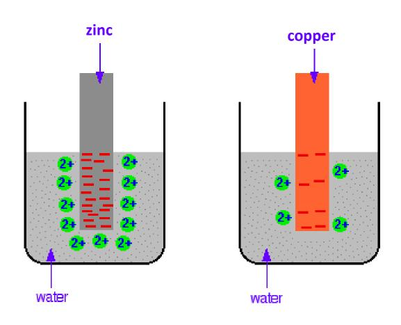
If we place two strips of metal in water then we can see the reactivity as indicated below. If we were to connect the two strips with a wire, then electrons could flow from the more negative to the the less negative strip.  $e^- \rightarrow$
