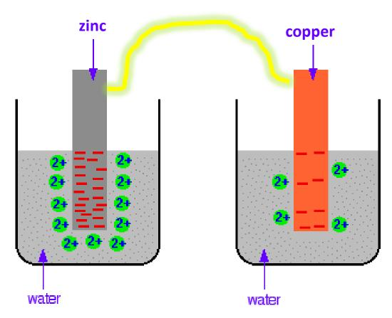
However, the electrochemical cell shown below does not make a complete circuit so the current would lead to a small net transfer of charge, and then it would stop.
