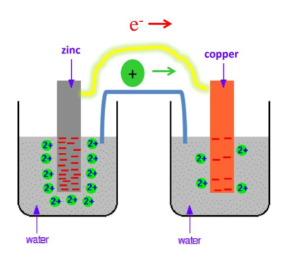
The process that we have described is the construction of an electrochemical cell. The two electrodes have different potentials, which sets up a cell potential.
